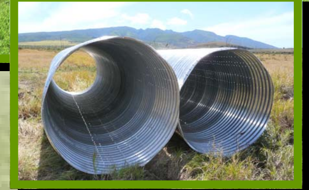
Photo Top - Original drainage swale used to capture off-site flows. Photo Middle - Location of the new subsurface D/R basin. Photo Bottom - 60-inch perforated corrugated aluminum drain pipes used for the subsurface D/R basin.
